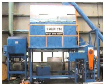
Wet-type gravity separator - Material recycling, pyrolysis oil, fuel (solid fuel) and localization
