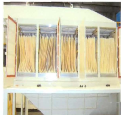
Photo of inner views of wet dust collector (MODEL: OILCOL-50000)
