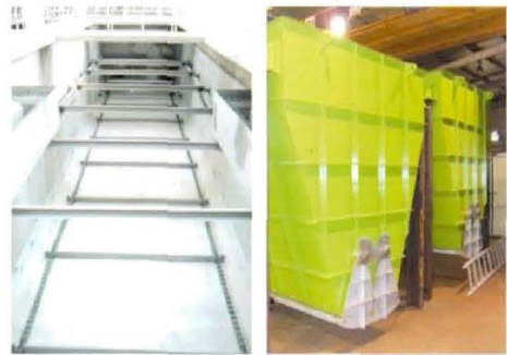
| Non-metal sludge collector & Hopper
